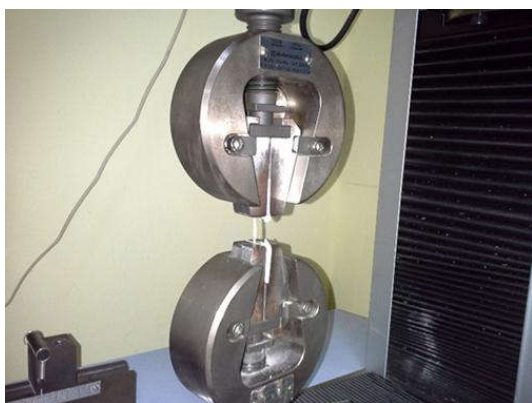
Plate 3: Tensile testing of kenaf fibres
